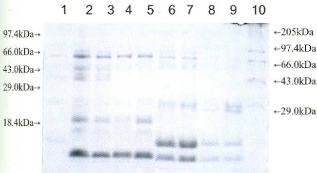
Fig-26. Comparisons of camel (M-13) and cow milk whey proteins denaturation during early lactation. Lanes 1 and 10: Marker; Lanes 2-5 of M-13 (lane 2: raw; lane 3: 63°C, lane 4: 80°C, lane 5: 90°C). Lanes 6-9 of cow (lane 6: raw; lane 7: 63°C, lane 8: 80°C, lane 9: 90°C)
